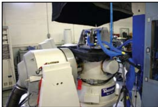
Figure 1 - Three-axis electrodynamic shaking, courtesy IMV, Visteon and Spectrum Technologies.
